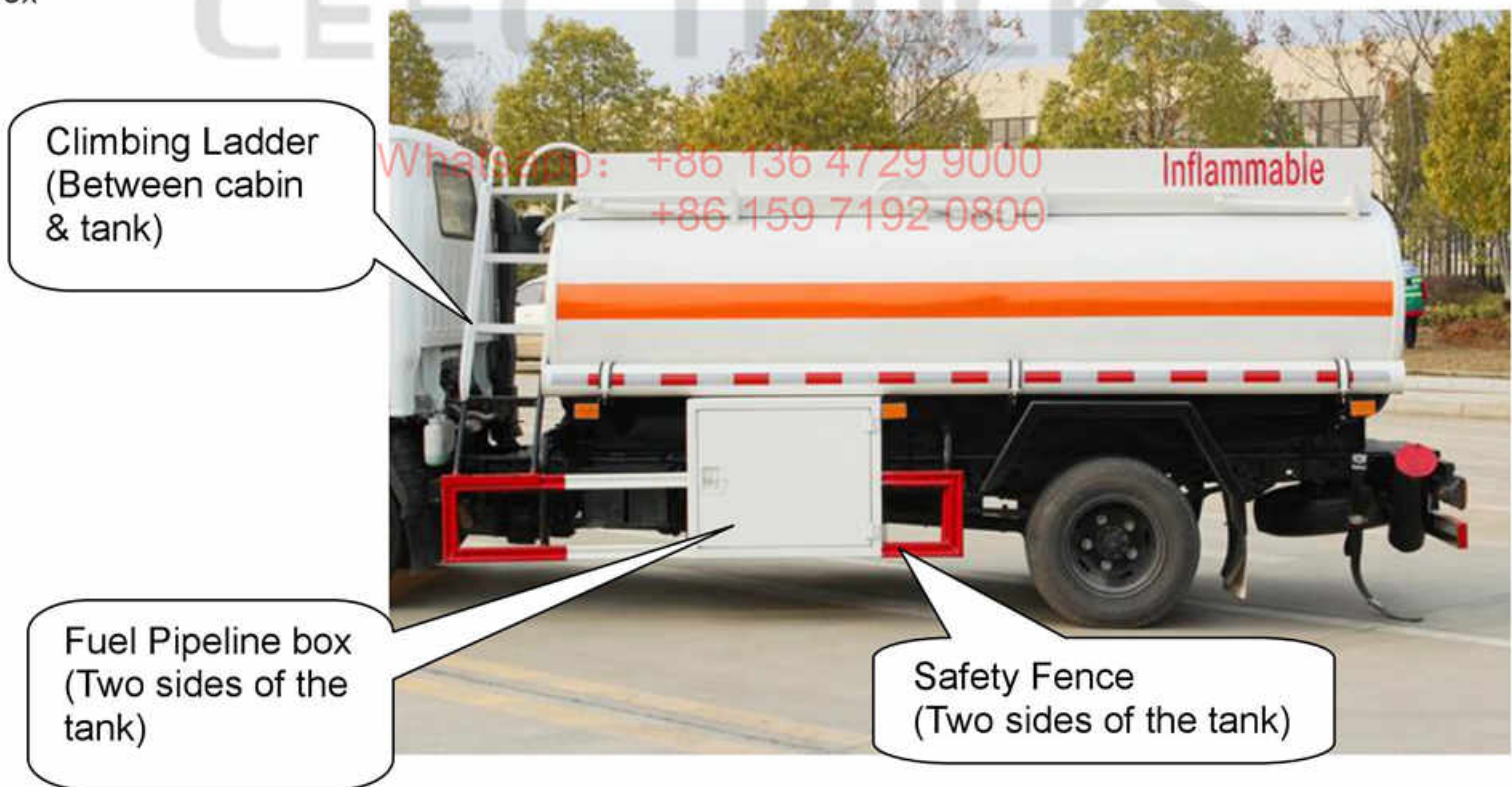
Side of the Tank: Climbing ladder with three level, Pipeline storage box & Fire-extinguisher storage box
